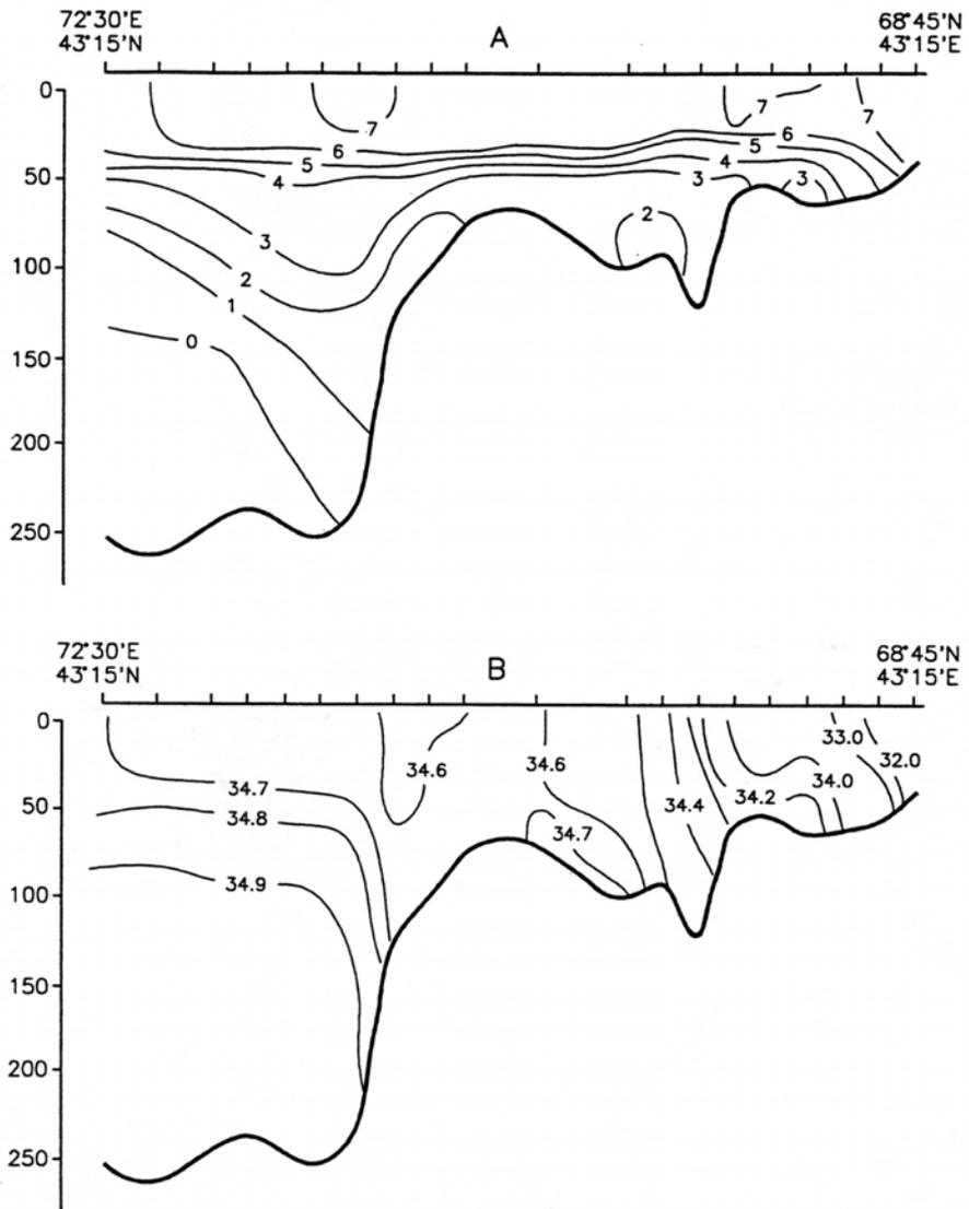
Fig. 15. Hydrographic section Cape Kanin-North. Temperature (A) and salinity (B)
