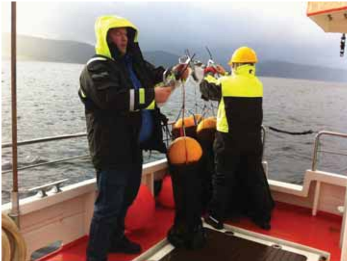
Figure 2.1. Mounting of GPS and dog collars to the drifters on board the Teist in Trondheimsfjorden.
