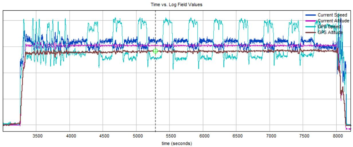
**Figure 9.** Altitude, airspeed and groundspeed from autopilot airpressure and GPS sensors. From the CW1 flight on 22 March.
