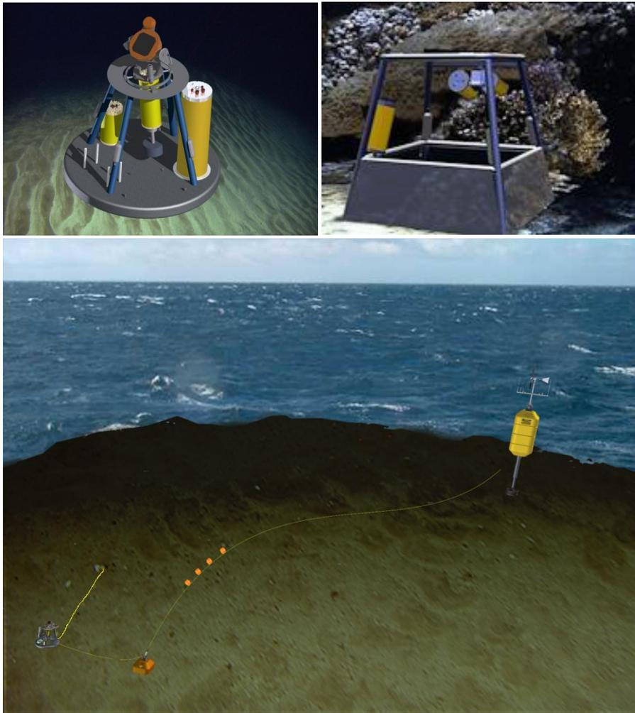
Figure 2 The acoustic lander, the camera satellite and the two connected to the surface buoy
