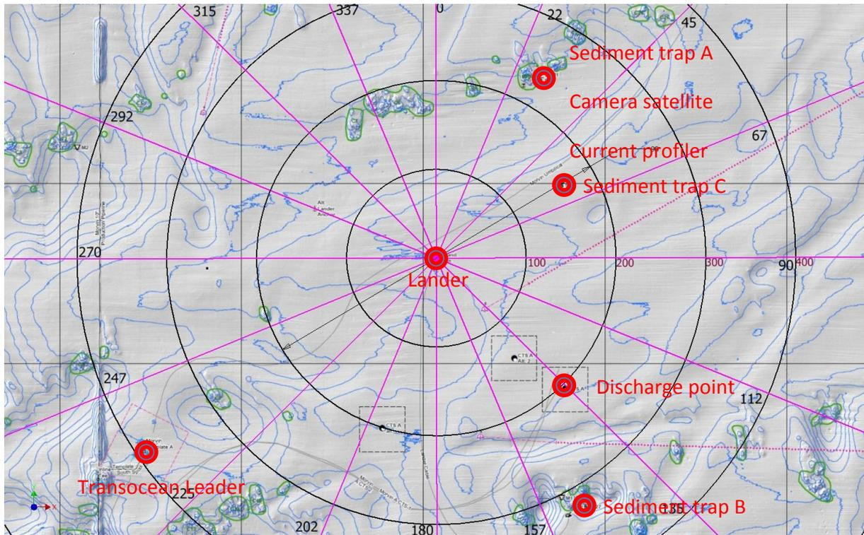
**Figure 2. Sediment trap positions during second drilling period (Feb 2010). Current direction was not measured successfully during the second drilling period so it is uncertain as to which traps were exposed to drill cutting material.**
