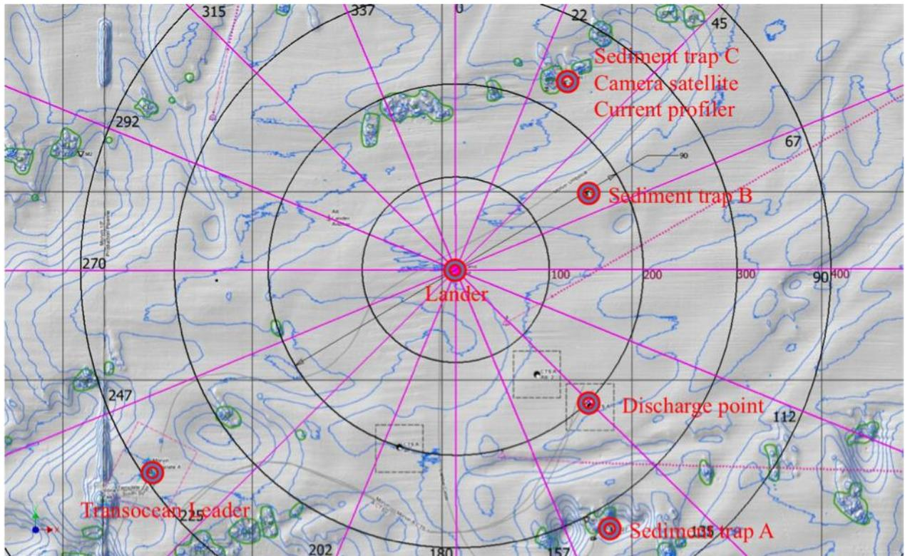
Figure 23. Sediment trap positions during initial drilling period (Nov-Dec 2009). Sediment trap A south and upstream of the discharge point and traps B and C north and downstream of the discharge point. Flow direction determined by current profiler, positioned close to sediment trap C.
