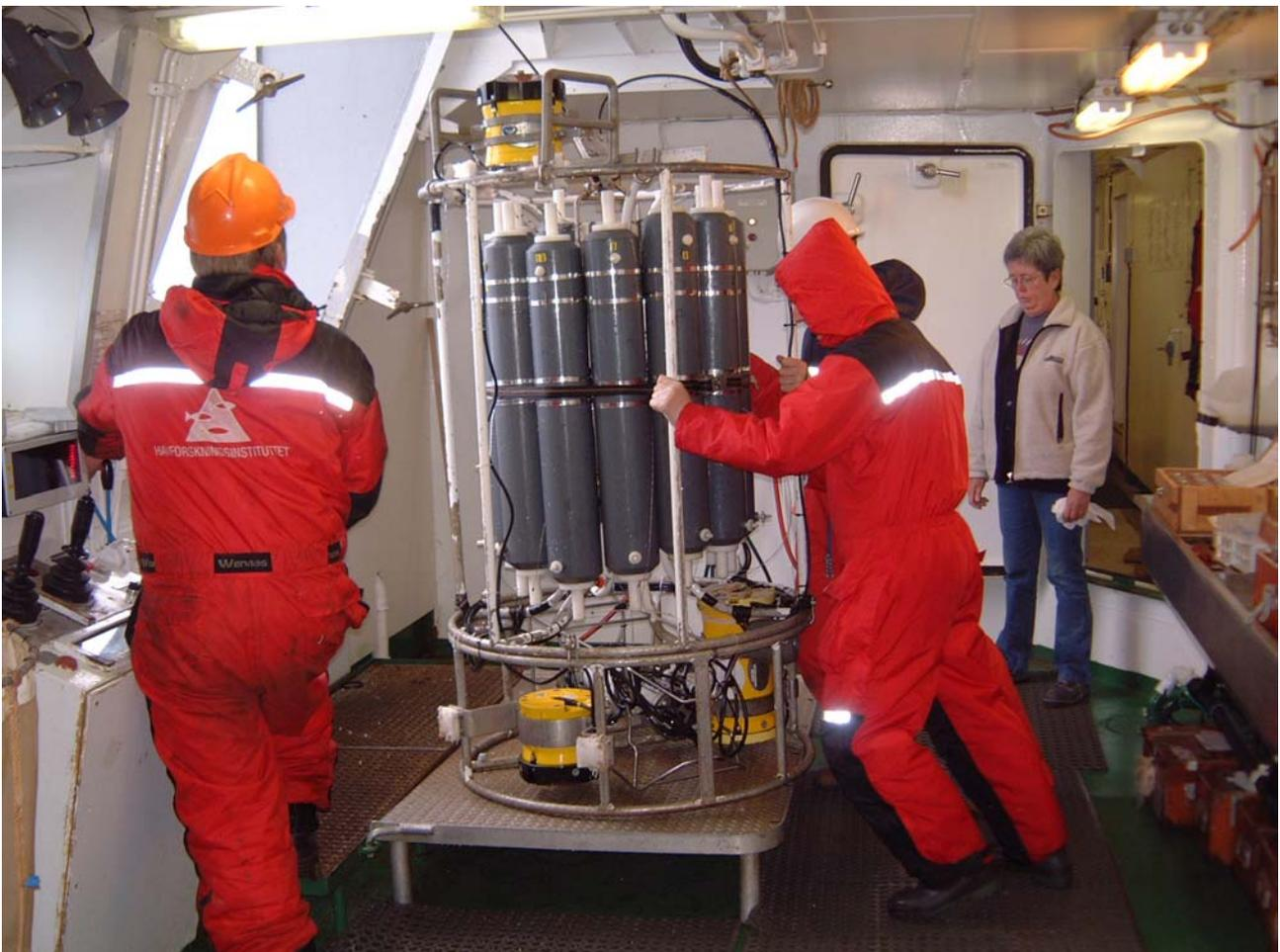
Fig.2 CTD probe used during the cruise
