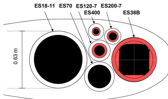
Figure 1. Relative positioning of transducers on protruding instrument keel of RV "G. O. Sars" (3)
