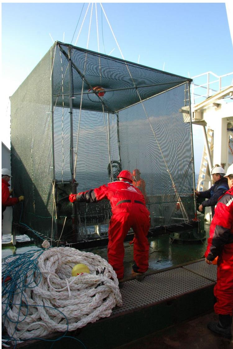
Figure. Net pen for in situ measurements of target strength of sandeel.
