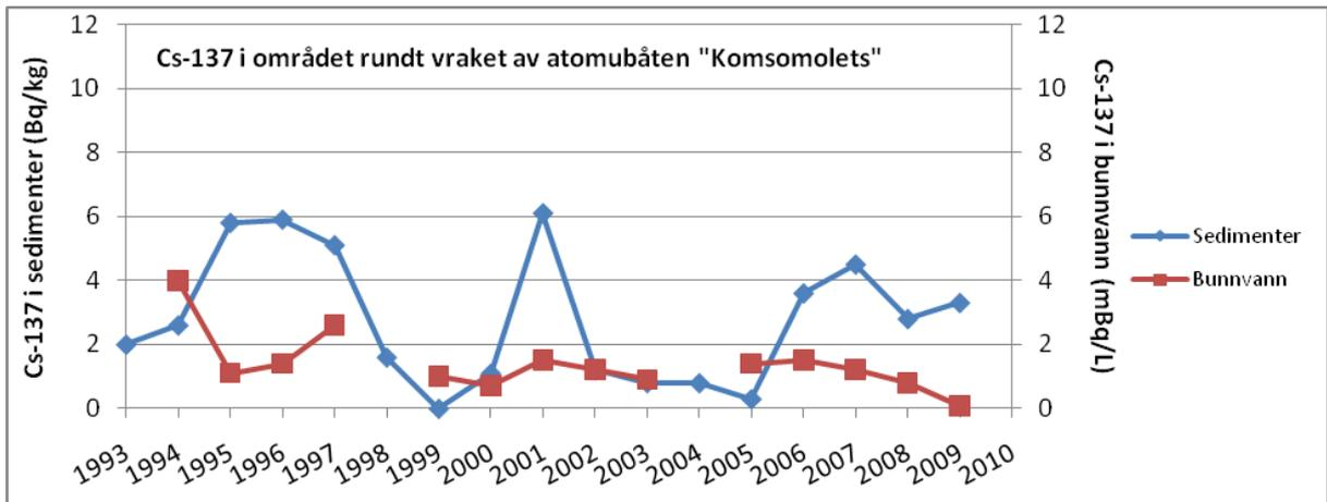
Figure 2.10.1. Levels of Cs-137 in sediments (left Y-axis, blue line) and bottom water (right Y-axis, red line) in the vicinity of the sunken Russian submarine “Komsomolets”. The submarine rests at a depth of about 1700 m southwest of the Bear Island.
