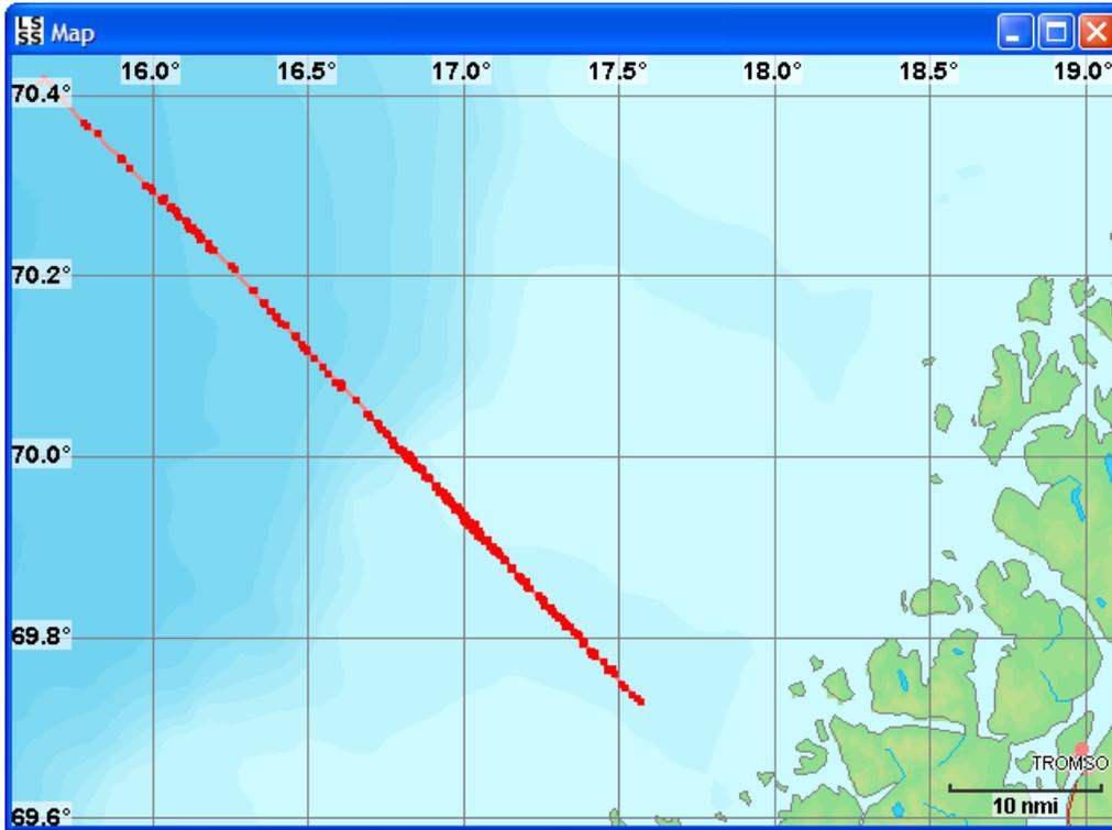
Figure 31. Schools detected by the SH80 sonar during the first survey transect during the second leg (26.07.2010). Each red dot represents the single detections for each school in every ping.
