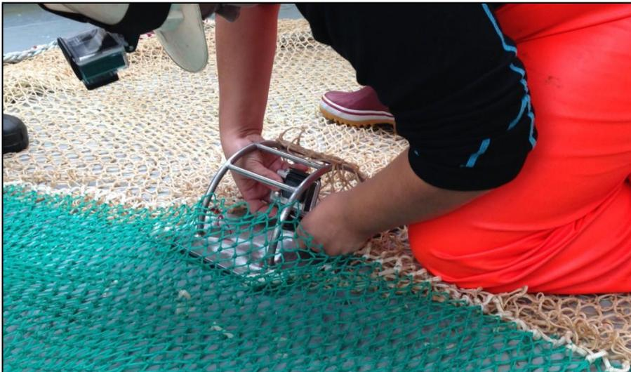
Photo 2. GoPro camera attached to inside of trawl by fish lock on Finnur Fríði. The steel frame was tied to trawl, at the each corner using a rope.
