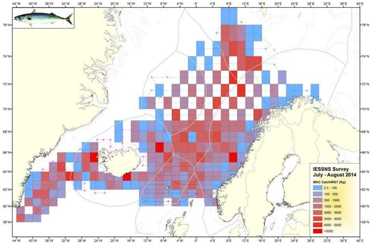
**Figure 12.** Catches of mackerel in kg represented in standardized rectangles. Light blue represents small catches (0.3-100 kg), while dark red represents catches of more than 5000 kg mackerel after 30 min standardized towing with the Multipelt 832 pelagic trawl. Vessel tracks are shown as continuous lines. Trawl stations are marked as small crosses for each vessel. Empty rectangles surrounded by three or more were interpolated in the calculations on biomass/abundance and density indices.
