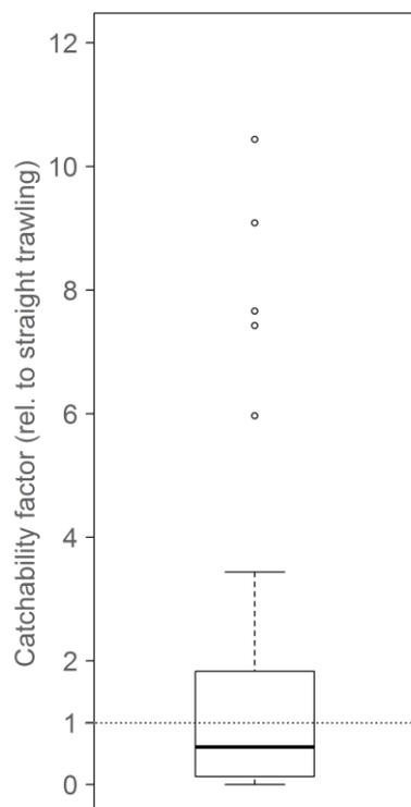
Figure 3. The effect of trawling method on the catch rate indicated by the Catchability Factor (*CF*). Boxes indicate the following quartiles: 25 %, 75 % and 50 % (median). Dots indicate outliers defined as observations that exceeded 0.67 times the quartiles. The whiskers indicate the most extreme observations, excluding the outliers.
