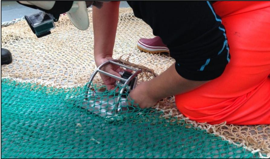
Photo 2. GoPro camera attached to inside of trawl by fish lock on Finnur Friði IESSNS 2014. The steel frame was tied to trawl, at each corner using rope.
