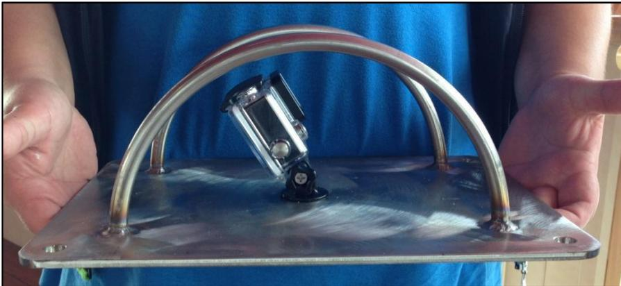
Photo 1. GoPro camera inside a waterproof box, mounted on steel frame and ready for employment in trawl on Finnur Friði IESSNS 2014.
