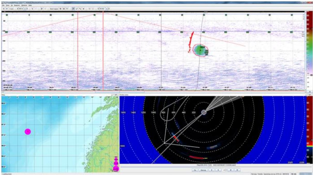
Figure 3. An echogram (upper panel) and sonar image (lower right panel) showing a herring school. The geographical location is shown in the lower left panel. The school was first detected by the sonar at 800 m, and later crossed by the vessel and measured with the echosounder.
