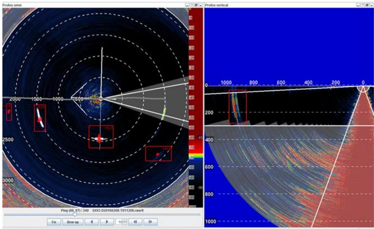
Figure 2. Sonar images of herring schools. Left panel: detected schools in the horizontal beams displayed with a white overlay and surrounded by a red square. Right panel: one school detected in the vertical beams. The same school was observed in the horizontal beams at a range of 1000 m on the port side of the vessel.
