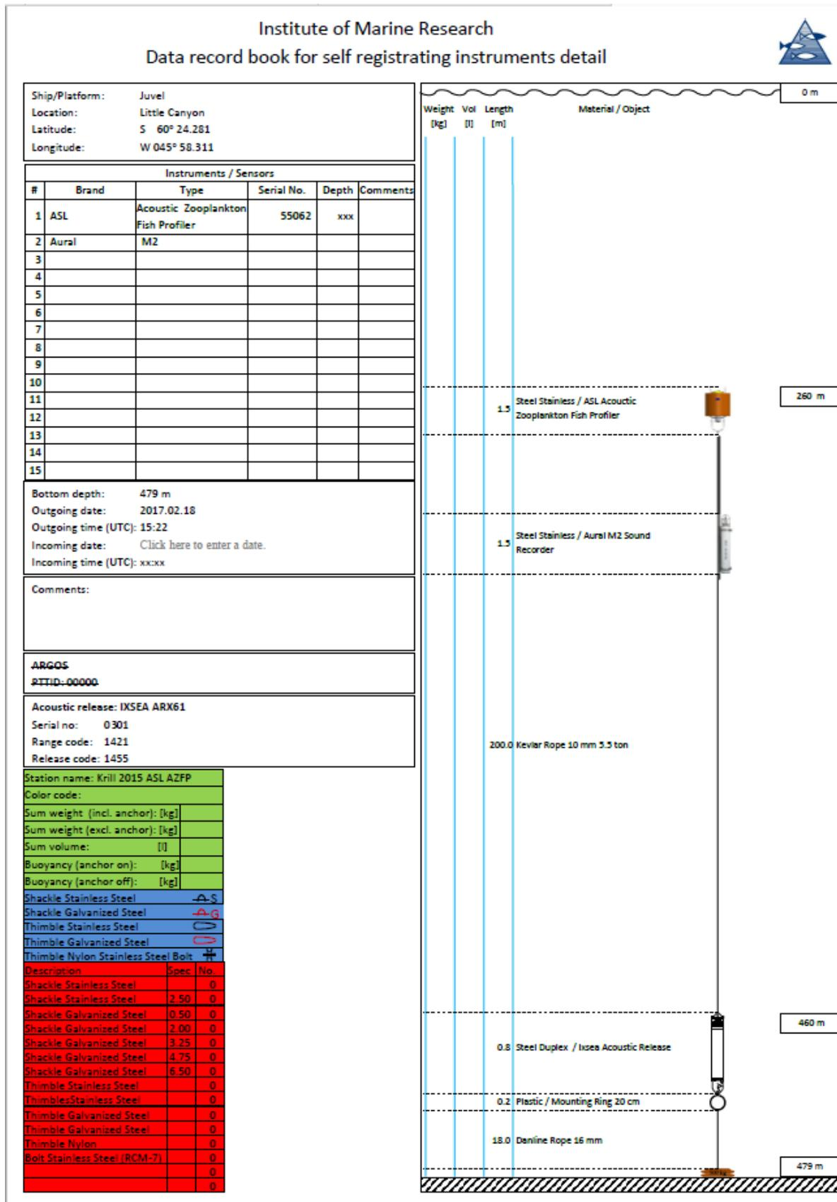
**Figure A1.** Details on the 2017 deployment of the ASL acoustic and AURAL sound recording moorings.
