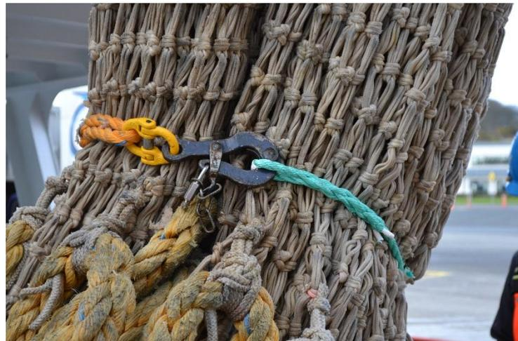
Figure 13: FossTech's prototype Catch Limitation Release (CLR). Left: CLR unit fitted to codend. Right: restrictor line and fastenings.
