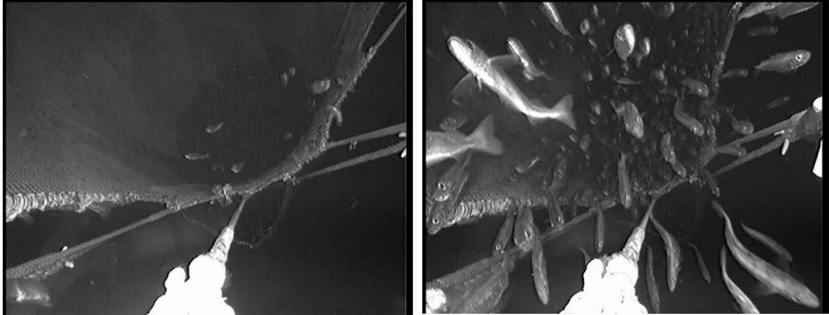
Figure 10 – Haul 09 (Rig 4) Fish-lock (type 2) fails to close during haul-back. Left: 17:15:05 – fish-lock open and loose in catch control rig. Right: 17:22:25 – fish swim out through fish-lock as codend ascends to surface.
