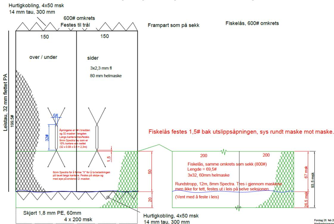
Figure 5c – Net Drawing of Catch Control Rig 3: 2.5m long slot, one in each of four Panels.
