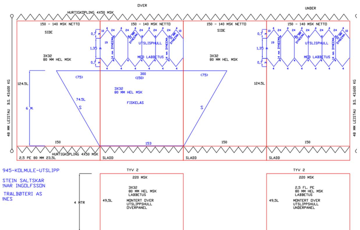
Figure 5a – Net Drawing of Catch Control Rig 1: 2.7m Hexagonal Meshes in Top & Bottom Panels.
