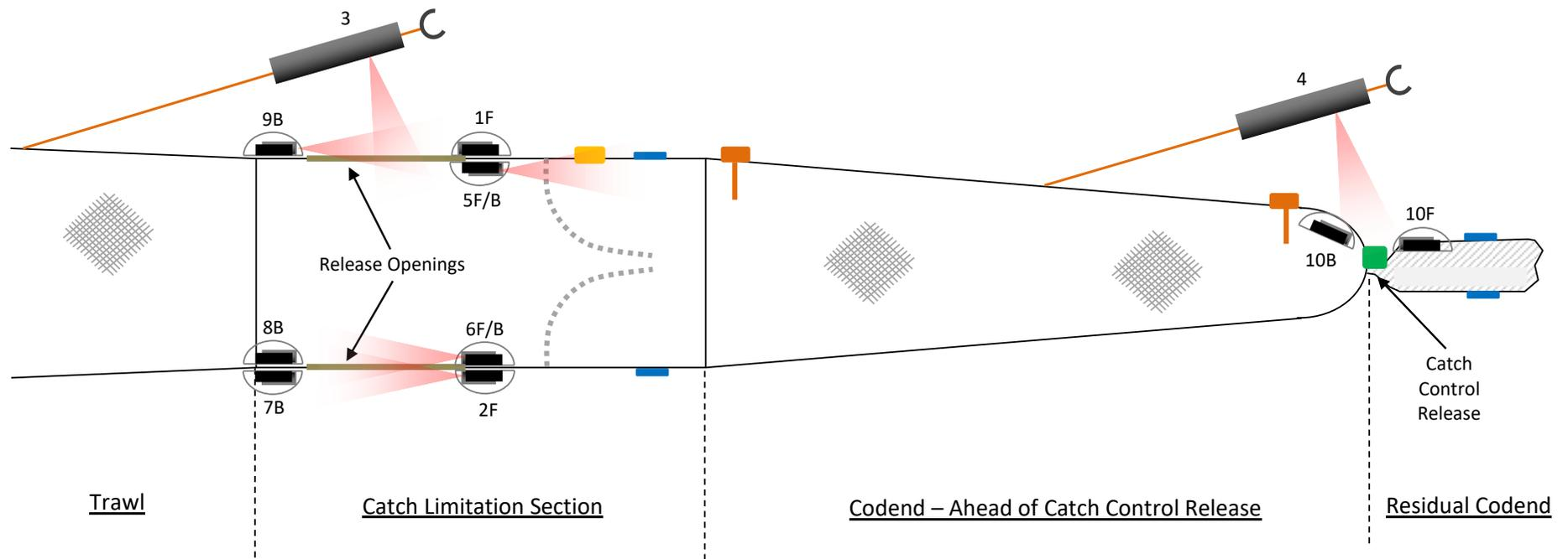
Figure A4 – Camera positions on the Catch Control Rigs and Codend. Post-script F means the camera was forward facing (toward the mouth of the trawl) and post-script B means the camera was backwards facing (towards the codend). The red shaded triangles provide an approximate indication of the illuminating light field in some example positions. See figures 4 and 12 for further explanation of the fishing gear components.
