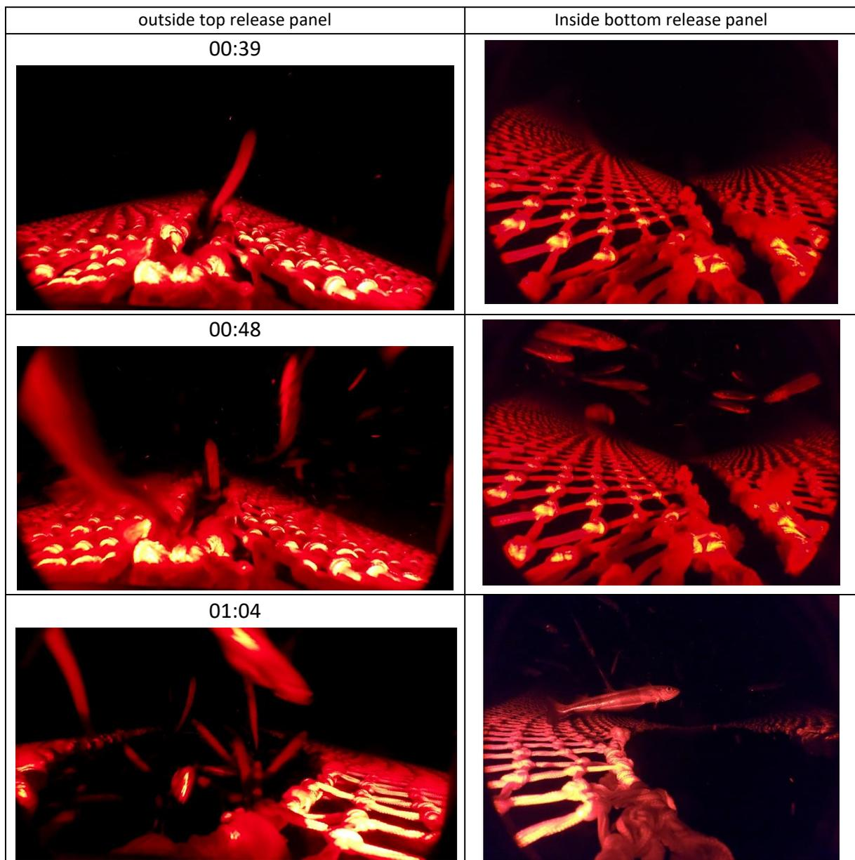
Figure 7 – Haul 07 (Rig 3). Left – outside top release panel; Right – Inside bottom release panel. Top: 00:39 – Haul-back starts; low density inside CCR; slots closed and few escapes. Centre: 00:48 – Sensor #4 on; density increases; slots begin opening; escapes increase in top panel. Bottom: 01:04 – 16min after Sensor #4 on; slots almost fully open; high escape rate in top panel, few escapes in bottom panel.
