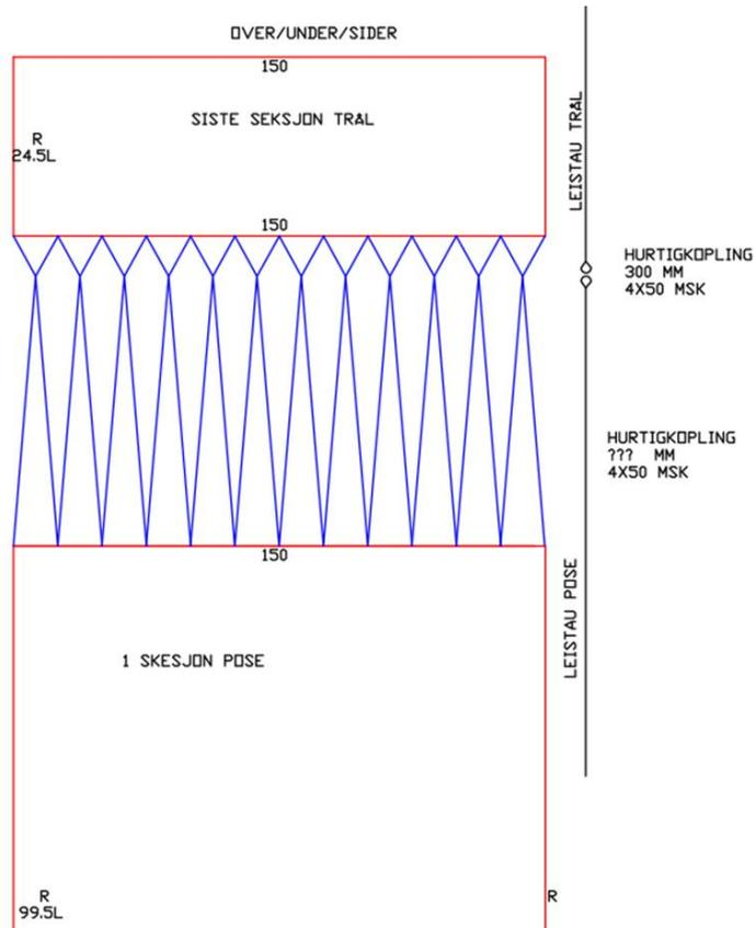
Figure 5b – Net Drawing of Catch Control Rig 2: 2.0m Meshes in all four Panels.
