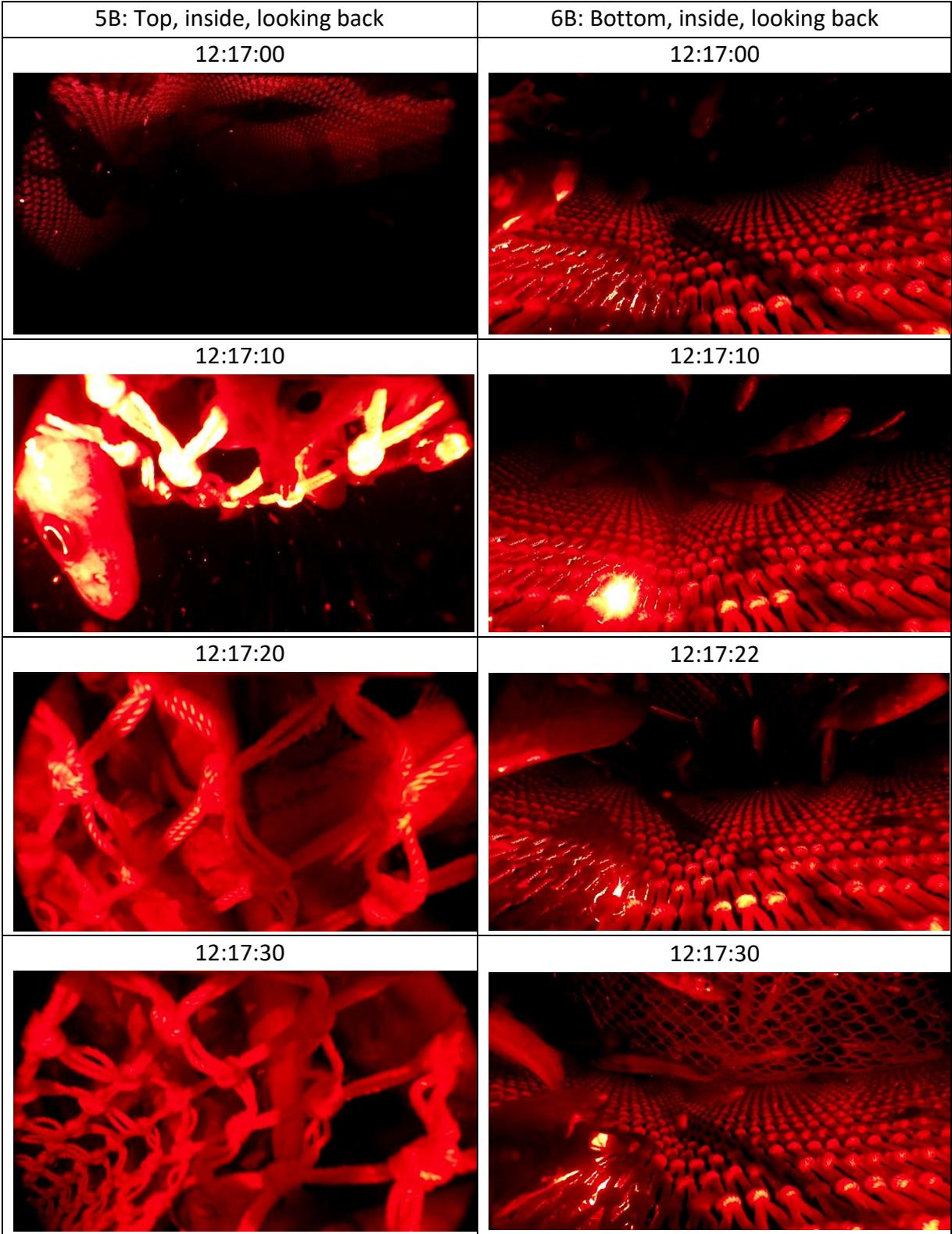
Figure 9 – Haul 03 (Rig 1b). Sequences of images of the fish-lock (type 1) successfully closing during haul-back. Left: Top panel looking back; Right: Bottom panel looking back.
