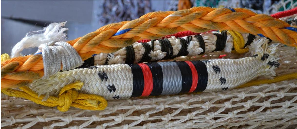
Figure 17 – a depth sensor (D-0130) in its protective housing and sheath fixed to the top of the CCR.
