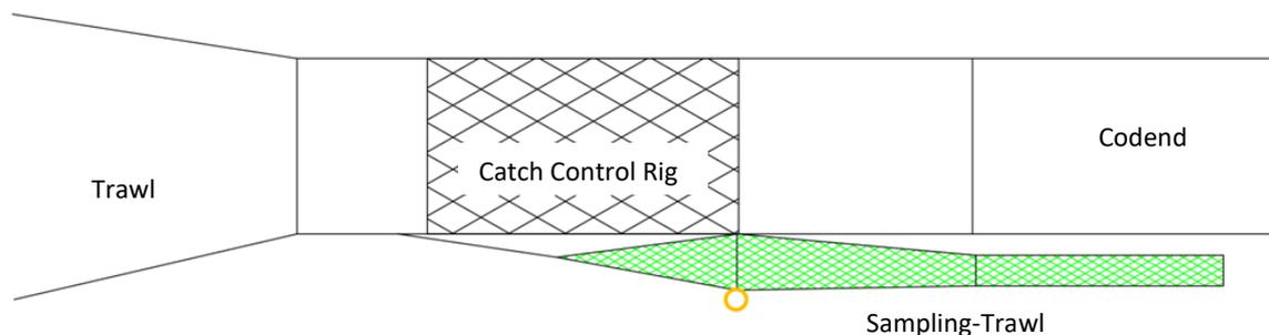
Figure 21 - Sampling-trawl beneath the catch control rig to collect fish released from the bottom opening.
