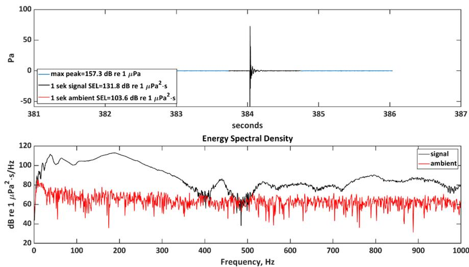
Figure 16. Example that also loud sounds can occur that is not seismic. This is a recording from the upper hydrophone at the array during block 2 in 2020 during the silent run. The frequency content of this pulse is however quite different from seismic.
