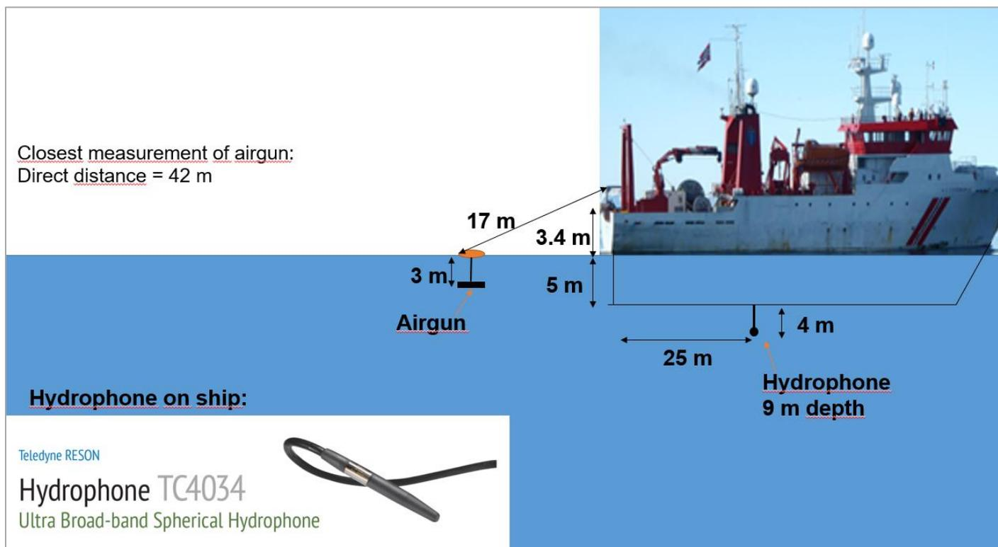
Figure 3. Air gun and hydrophone set up at H.U. Sverdrup.
