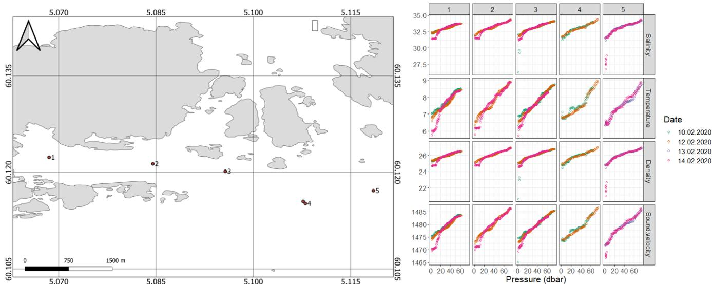
Figure 6. CTD casts for 2020. Casts are taken at the same five positions, but repeated throughout the week (details in table 5). Left: Locations of the CTD stations at positions of the inner (1) and outer (3) bottom hydrophone rigs, the hydrophone array in the middle of the bay (2) at the center of the racetrack (4) and outside the racetrack (5). Right: CTD profiles for the 5 locations, with different colors representing different sample days.
