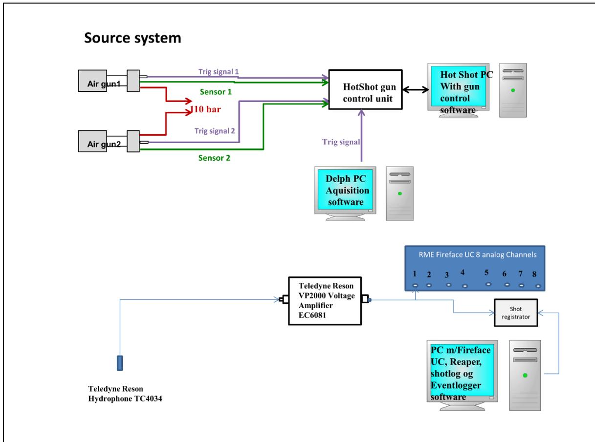
Figure 4. The exposure system and the vessel mounted hydrophone.
