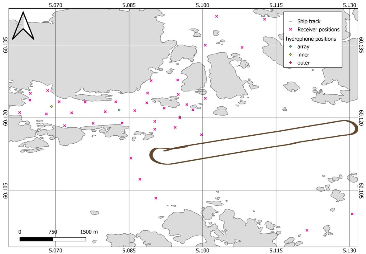
Figure 5. The 3nmi racetrack sailed by the source vessel (HUS) during the seismic and no-seismic exposure sessions. During silent control sessions HUS stayed in a holding area south of the exposure site sheltered from the cod spawning site. The hydrophone bottom rigs (inner and outer) and hydrophone arrays, as well as the Vemco receivers are also marked in the map.
