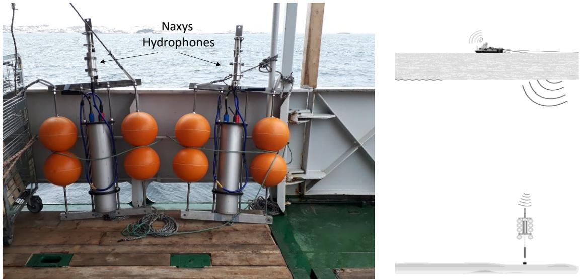
Figure 9. The two hydrophone platforms onboard HUS, ready to be deployed (left) and a figure of how it looks when deployed (right).
