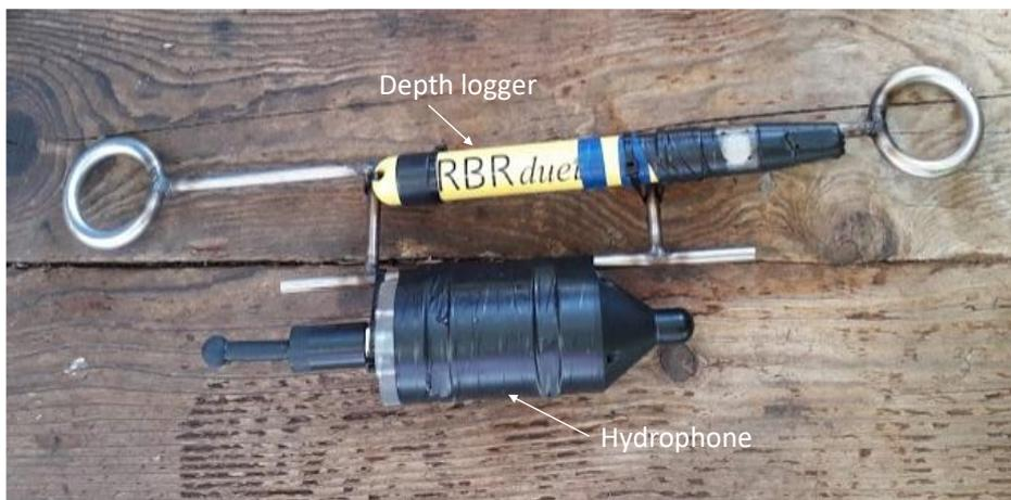
Figure 10. The sound trap hydrophone.
