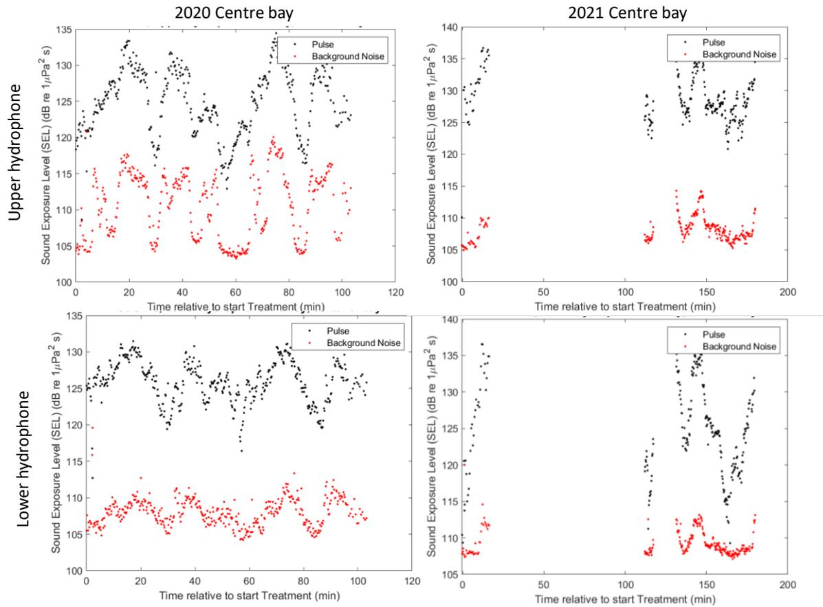
Figure 14. Sound Exposure Levels for The vertical hydrophone array in the centre of the bay, with two hydrophones at different depths at the same location; one at 8 m (upper hydrophone) and one at 37 m (lower hydrophone). The example for 2020 are from block 2 and for 2021 from block 11. For 2021, some of the data are missing due to this hydrophone being somewhat unstable in its recording, causing such datagaps.
