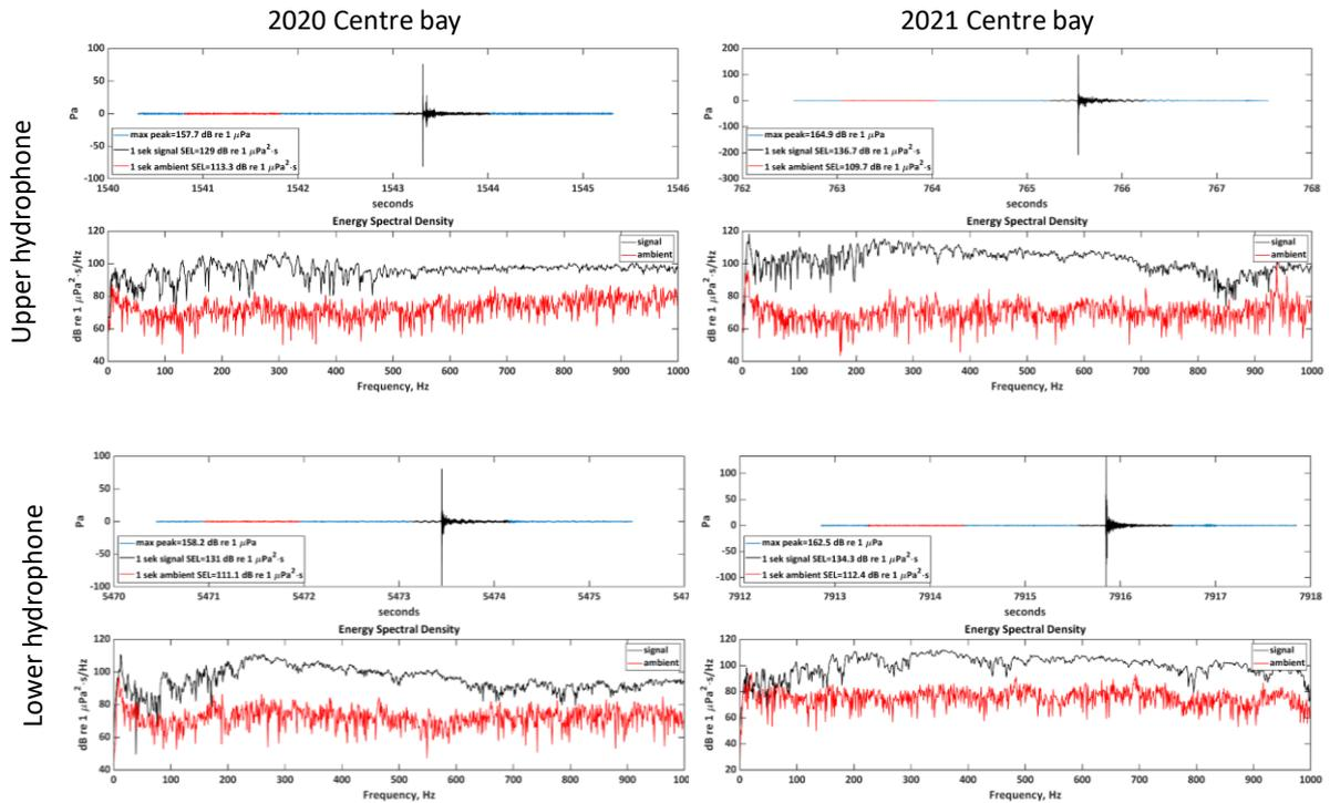
Figure 15. Examples of some selected pulses from where the frequency of the pulse and of the background noise is analysed for the vertical array hydrophones. The upper level of each plot shows a seismic pulse in black, as well as a similar interval of the background noise in red. Below in the spectral level of the seismic pulse and the background noise. Data from 2020 are from block 2, and for 2021 from block 11.
