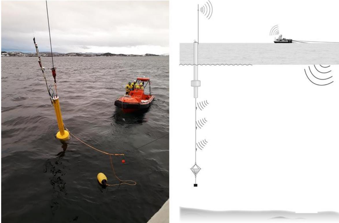
Figure 8. The hydrophone vertical array. Left: The surface part of the array visible above sea level. The array was towed by the HUS workboat into position, and moored to the bottom with heavy weights. Right: figure of how it looks when deployed. The figure shows 3 hydrophones at different depths, but in the current setting only two were used and the array was not drifting but fixed at one position.
