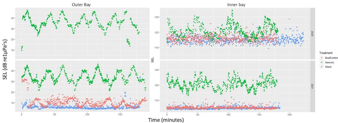
Figure 11. SEL for the three different treatments (seismic, silent, boat control) for the two years for the outer (left) and inner (right) hydrophone. For the outer bay, data for control runs (boat, silent) are not available. The figures are based on the data from the blocks indicated in green in table 13. All pulses are not included because only 22 of 30 seconds was recorded. Pulses in the centre of the recording was selected.
