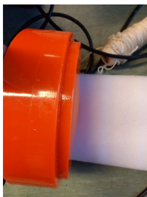
Figure 1. Picture of damaged transducer with convex shape in the transducer face.
