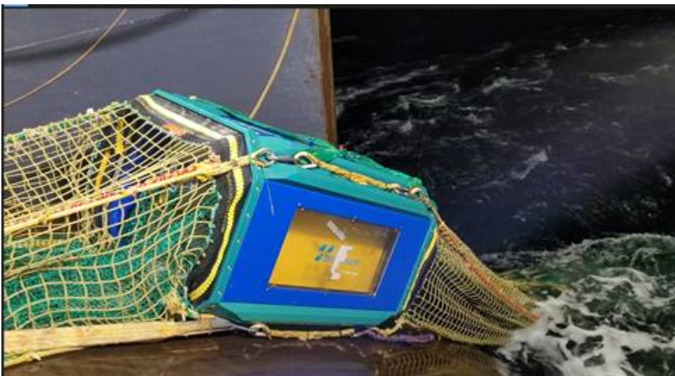
Figure 9. Deep vision is an open trawl where the catch goes through a camera tunnel before it goes through the open cod end of the trawl. It is used in research to document what is in the different acoustic layers without having to catch the fish. It is developed by Scantrol in collaboration with IMR. Picture by K. de Jong.
