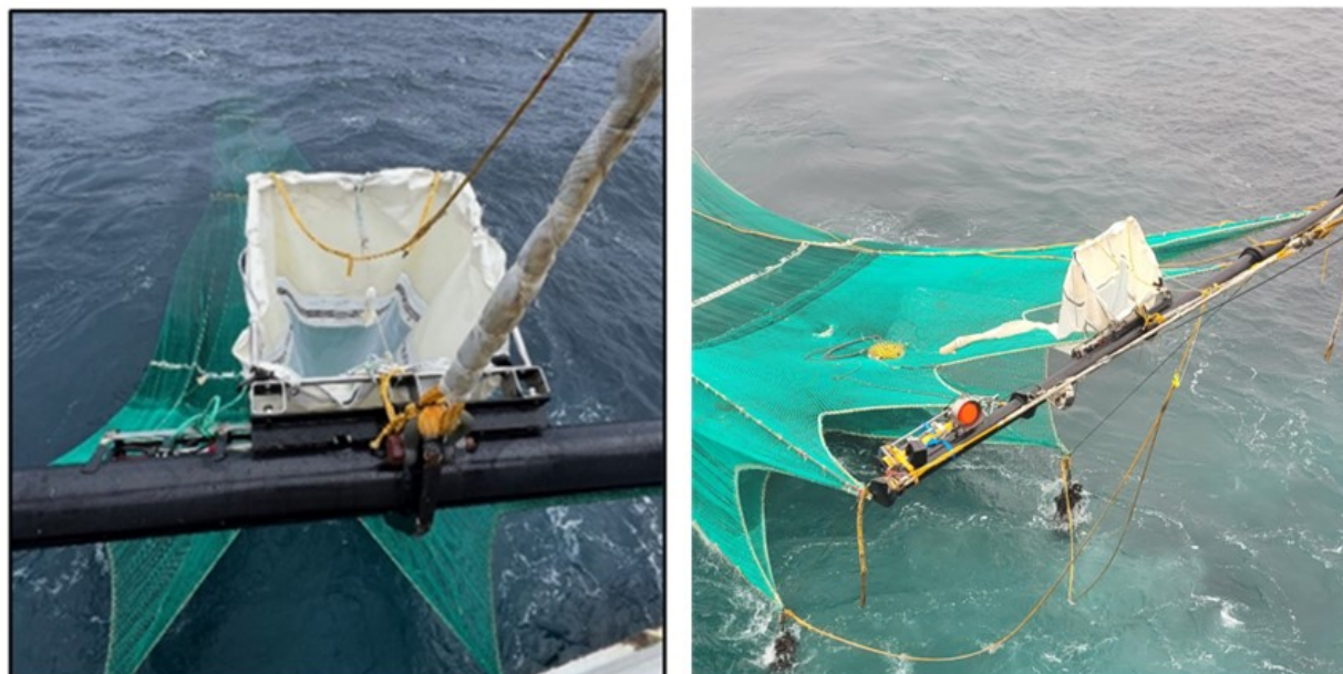
Figure 7. Trawl with a 180 \mu m plankton mesozooplankton net on the trawl beam, with mechanical flowmeter in the mouth. The right-side figure also shows the location on the beam with the SIMRAD Transceiver (WBAT) and forward-facing 120 kHz transducer.
