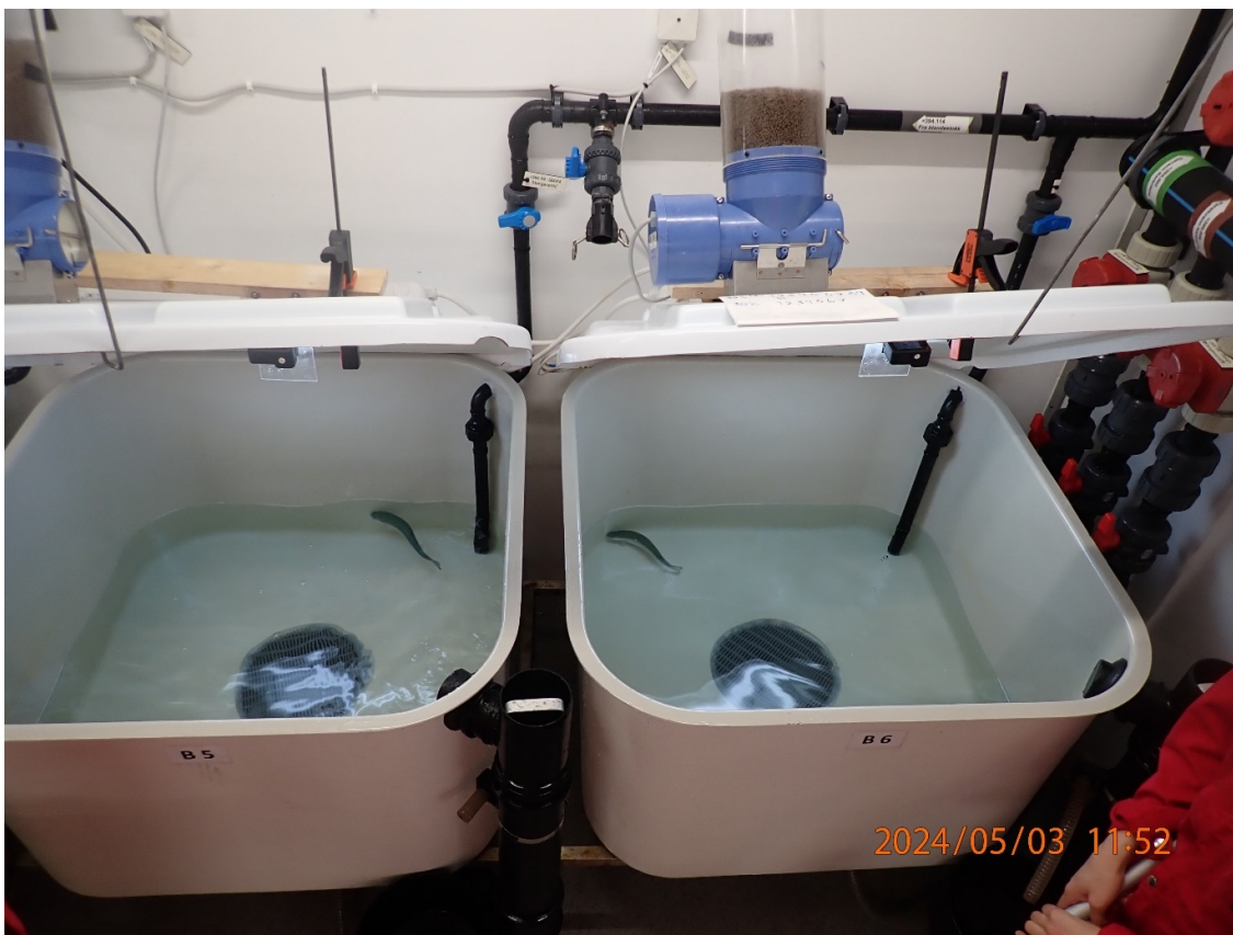
Figure 5.1. The tanks used for thermal exposure of small rainbow trout.
