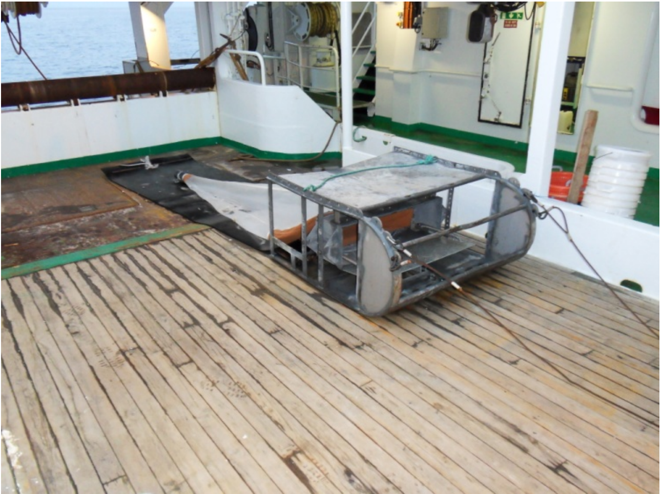
Figure 5 The RP sledge equipment used in MAREANO for collecting hyperfauna samples
