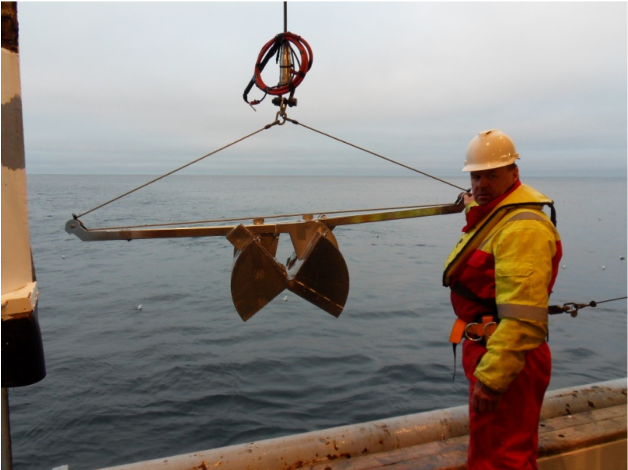
Figure 3 The 0.1 m 2 Van Veen grab, used in MAREANO for collecting sediment, including infauna, samples
