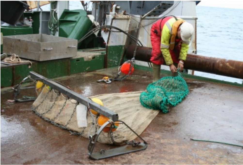
Figure 4 The beamtrawl equipment used in MAREANO for collecting epifauna samples
