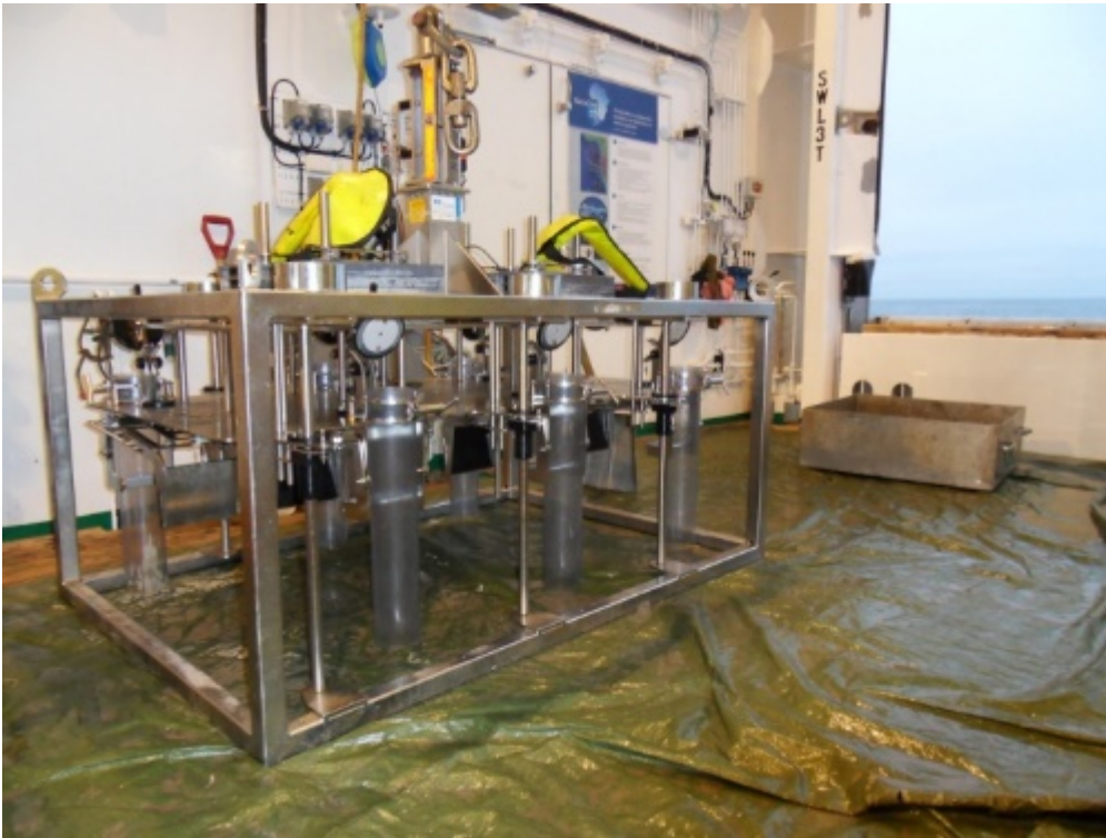
Figure 1 The multicorer equipment used in MAREANO for collecting chemical samples
