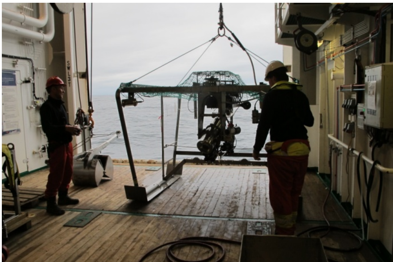
Figure 6 The towed camera system Chimaera, used in MAREANO to capture video footage of the seabed
