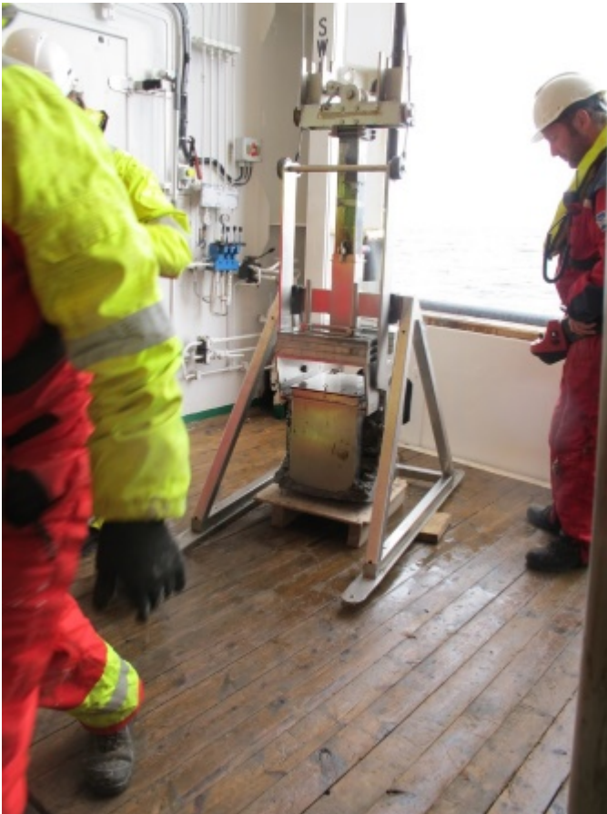
Figure 2 The boxcorer equipment used in MAREANO for collecting sediment samples to measure grainsize as well as ancillary biological parameters
