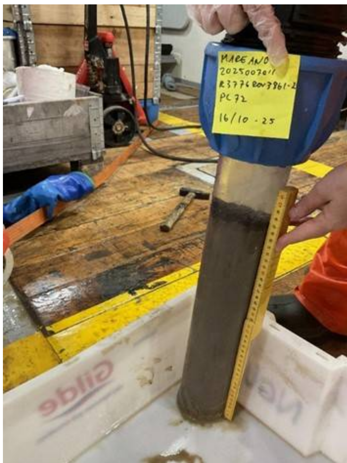
Photo 3. Example of an external push corer photo once on board. Photo by Geological Survey of Norway.
