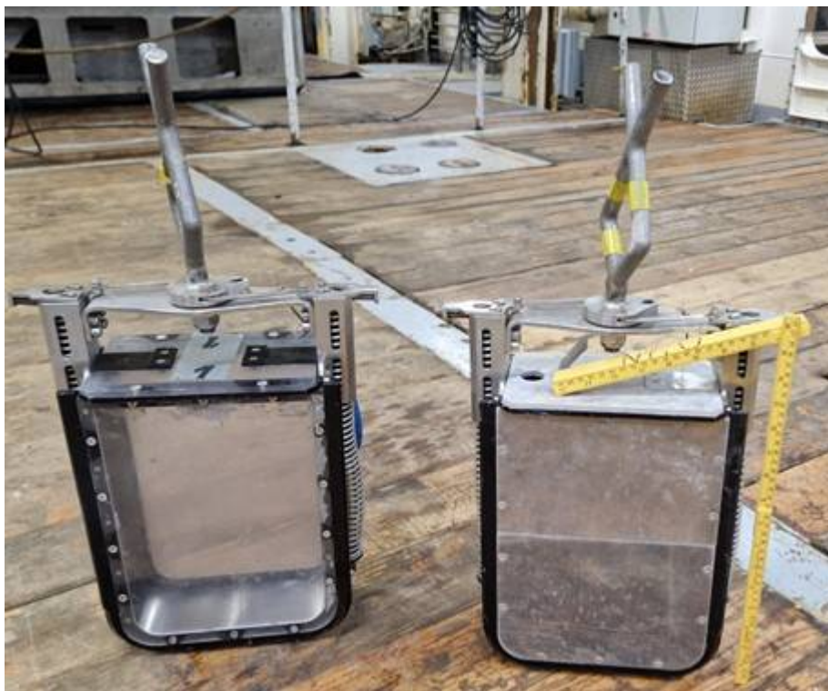
Photo 5. Side-by-side photo of the blade corers with plexiglass plates (left) and aluminum plates (right).
