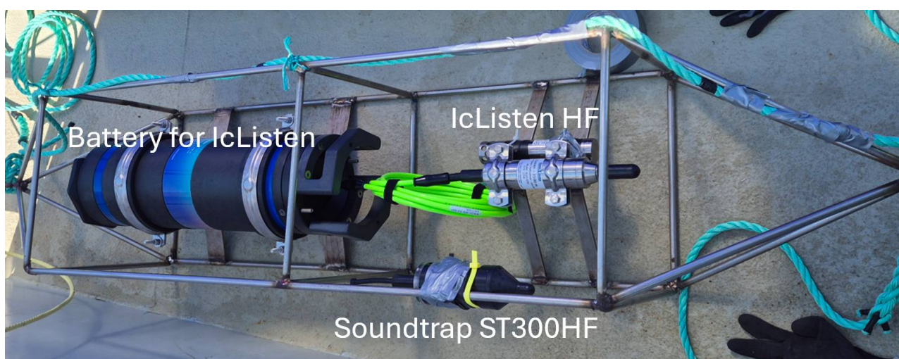
Figure 4. Hydrophone rig in the centre of the bay. The IcListen hydrophone required a large battery pack which was mounted in a steel frame. A sound trap hydrophone was also mounted on the frame. A depth logger (Starmon TD) is attached next to the IcListen hydrophone.
