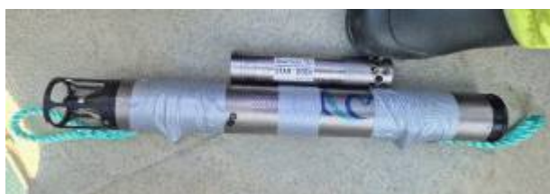
Figure 5. SoundTrap ST600STD and depth logger
