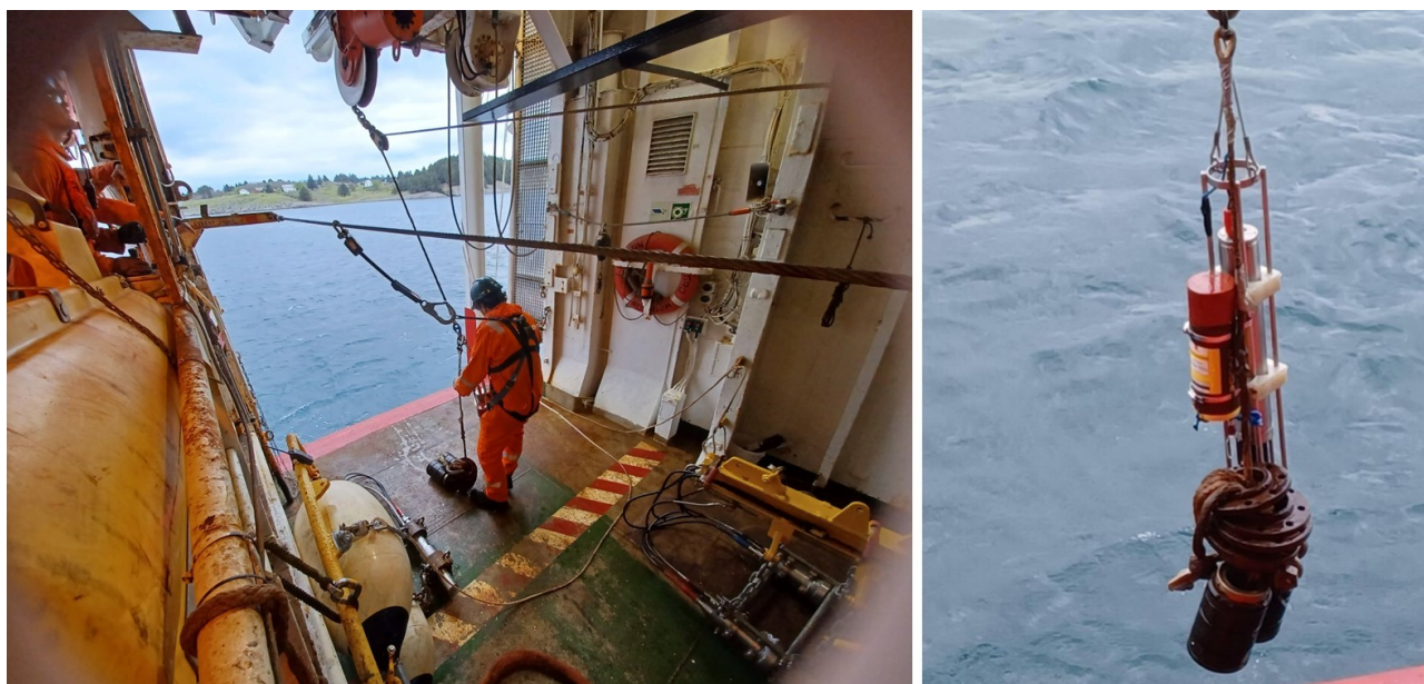
Figure 6. The CTD instrument about to be deployed (left) and close up before being submerged (right).
