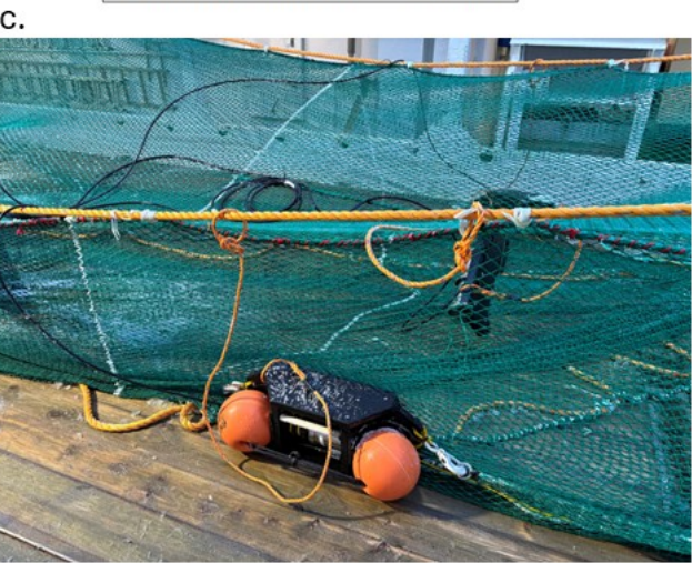
Figure 26. ActSel (Rose and Barbee, 2022) is a by-catch reduction device that can quickly be altered between capture and release configurations with real-time triggering. An electric actuator controls a water kite that moves a fish-guiding net panel. Panel design (a), kite (b), actuator (c) and the stretch release used to reduce load on the 3rd wire (d).
