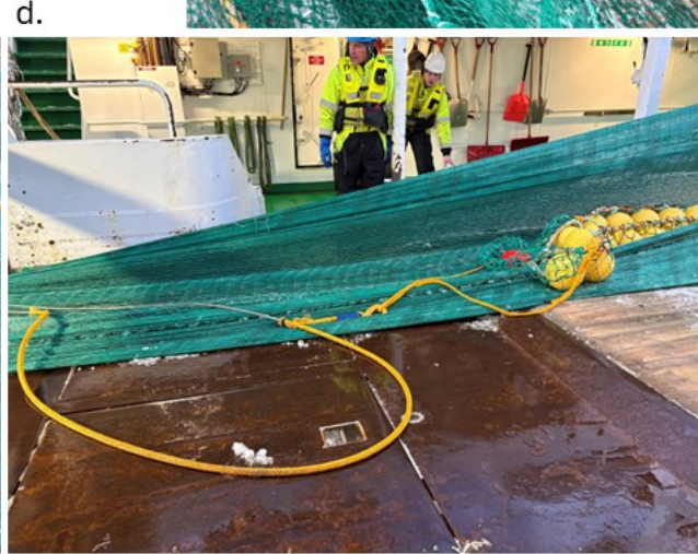
Figure 26. ActSel (Rose and Barbee, 2022) is a by-catch reduction device that can quickly be altered between capture and release configurations with real-time triggering. An electric actuator controls a water kite that moves a fish-guiding net panel. Panel design (a), kite (b), actuator (c) and the stretch release used to reduce load on the 3rd wire (d).
