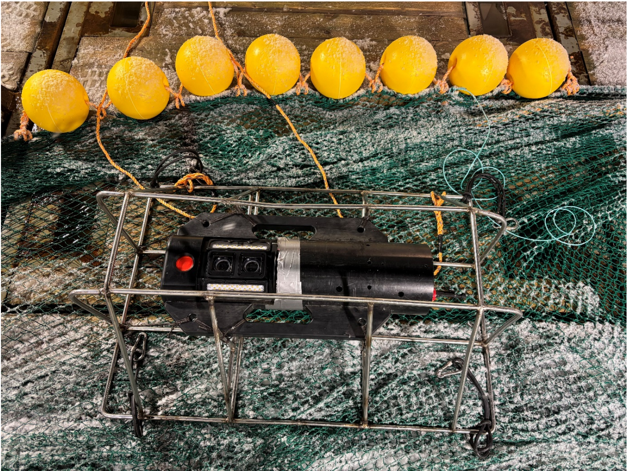
Figure 20 . The CamSounder was mounted in a protective steel frame on the starboard side panel of the trawl.
