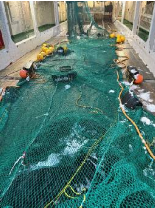
Figure 28 . Extension section with the ActSel system showing the actuators, kites, lines going from the actuator to the kite, Simrad live cameras, the FX hub and CamSounder.
