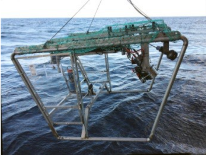
Figure 1: The video rig 'Chimaera' equipped with several video cameras, laser pointers for size measurement, transponders for positioning and CTD.
