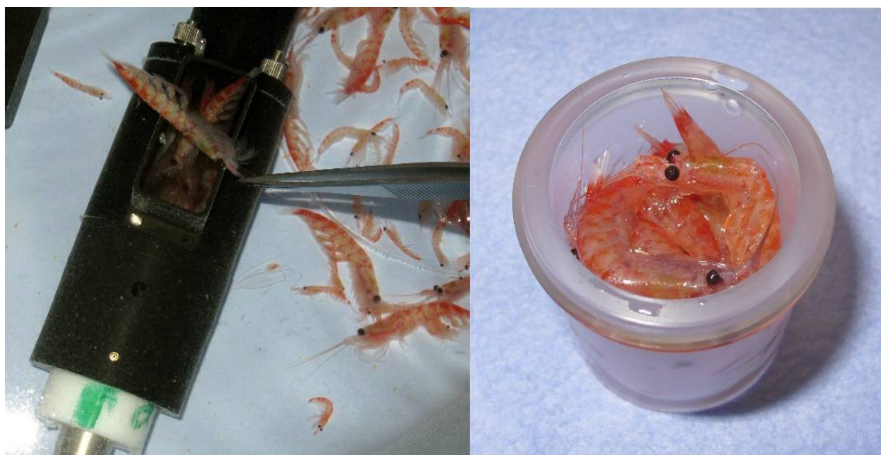
Figure 13.1. Krill being placed into the submerged sound speed measuring chamber (left image); krill in the container ready for weighing.
