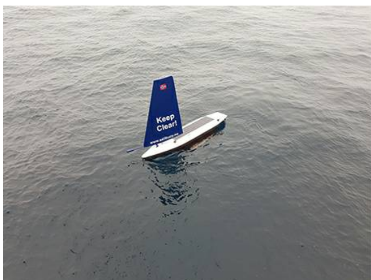
Figure 11.1. The Sailbuoy autonomous surface vehicle (left) and the transducer mounted in a gimbal in the keel (right).
