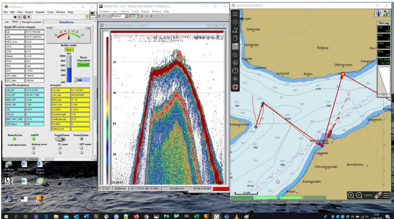
Figure 5. Screen dump of the kayak drone PC. To the left is the EchoDrone.exe control software. In the middle EK60 software showing a school of sprat in the current position close to the shore. To the right is the OpenCPN chart program. The route is indicated by consecutive red arrows. Next waypoint is indicated by a red circle with yellow fill. The drone is shown as a red ship and the actual sailed track of the drone is shown as a curved line.
