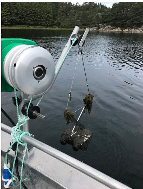
*Figure 2. Van Veen Grab sediment sampler.*
