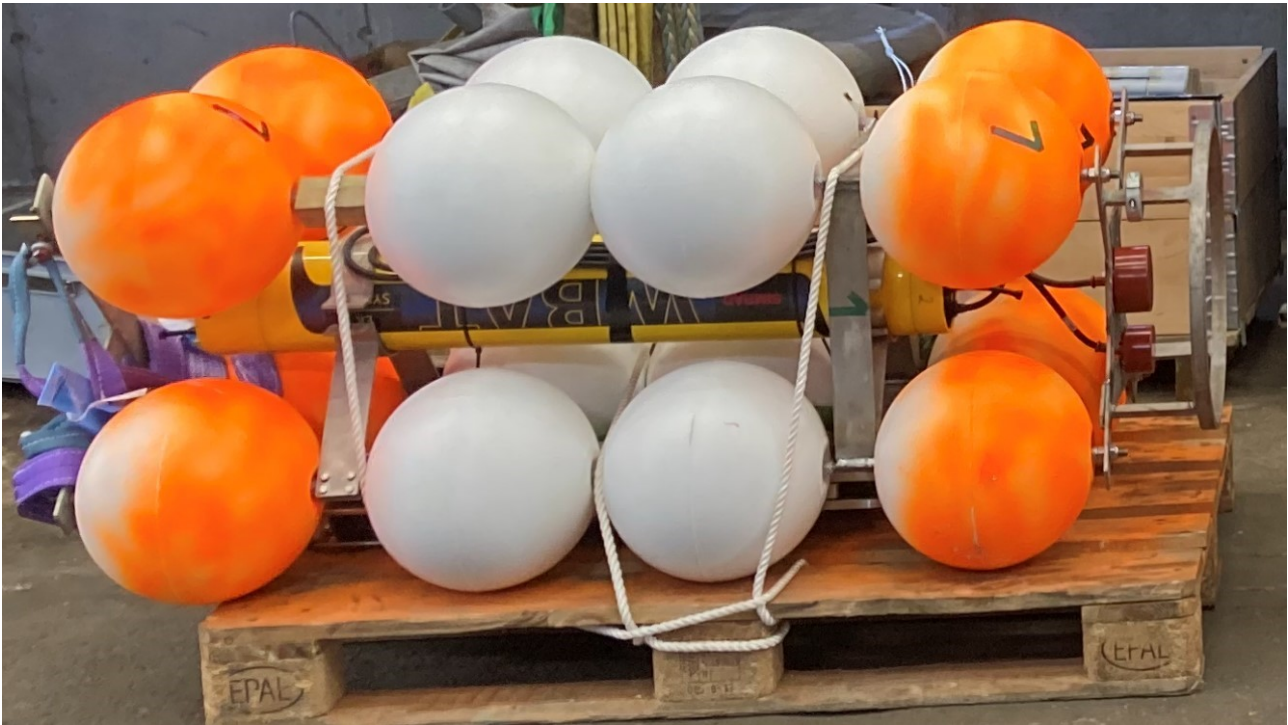
Figure 3. WBAT (wide band transceiver) with to upwards looking transducers. Picture by Anne Christine Utne Palm.
