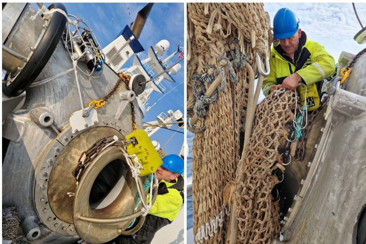
Figure 7.3 – Left: releaser and securing chain (Rig A) attached to pump-head, without the cod-end skirt attached. Camera and depth-sensor array is in a protective steel frame at the top of the image. Right: releaser and securing chain (Rig A) with the cod-end skirt fitted to the pump-head, showing the release jaw side of the releaser.
