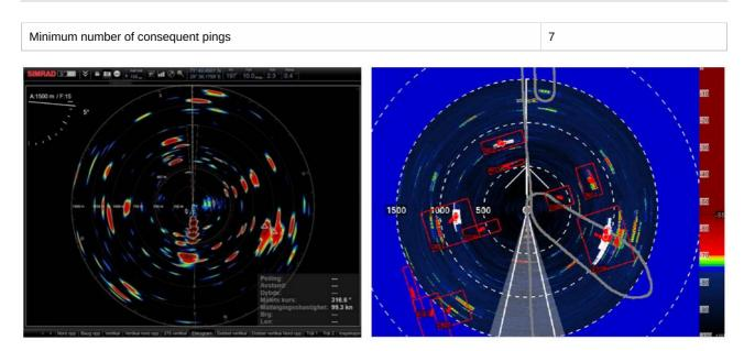
Figure A1. Example of a situation where a large number of small schools are detected with the sonar. To the left is a screen dump from the sonar and to the right from PROFOS (LSSS).
