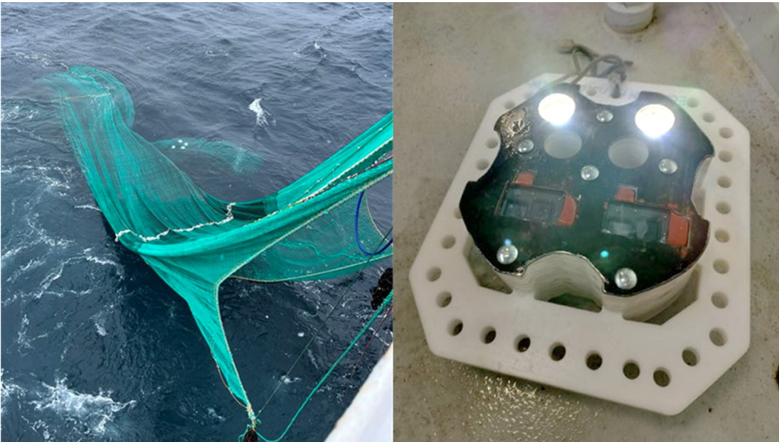
Figure 8. To the right (A): Stereo camera consisting of a specially made housing for fixating underwater lights and GoPro cameras. To the left (B): The installation of the camera in the survey trawl is visible by the added four white floats forward of the codend.
