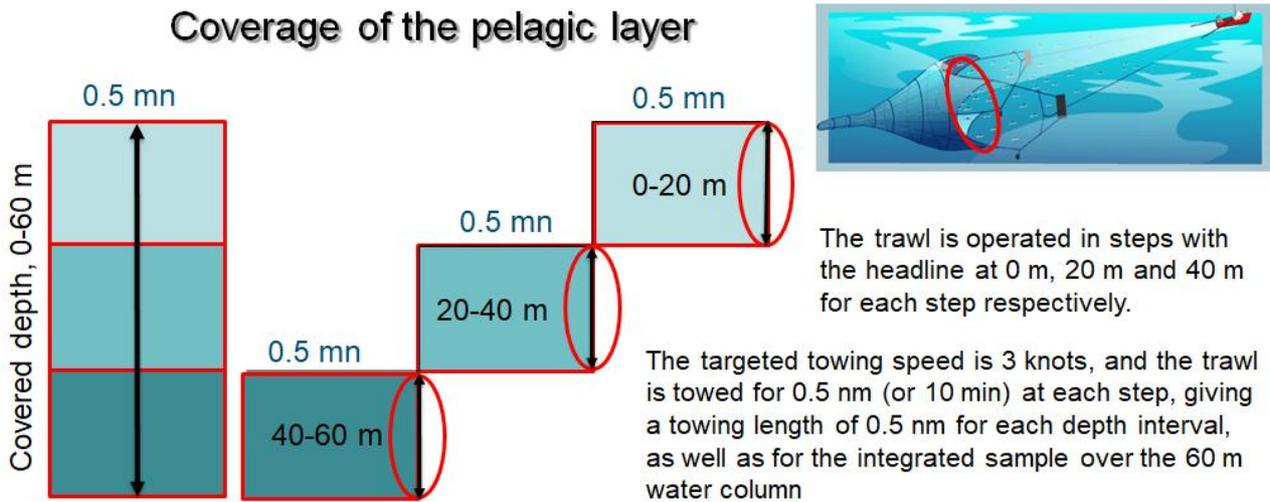
Figure 2. Schematic representation of a pelagic trawling (standard 0-group trawling), indicating three depth steps with headlines at surface (0 m), 20 m and 40 m. With a theoretic trawl opening of 20x20m, this provides an integrated sampling over the upper 60m water column .
