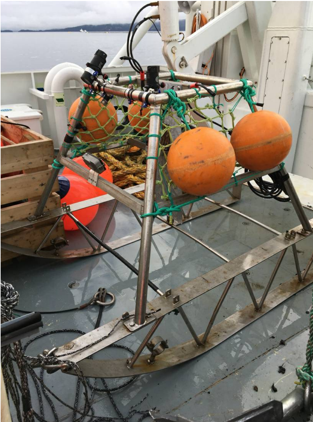
Figure 6: The video sled used for counting Nephtys burrows in the bottom sediment in the 2023 survey in Vestlandet. The two cameras (black) are mounted on top of the sled, one facing forward and one facing perpendicular to the sea floor.
